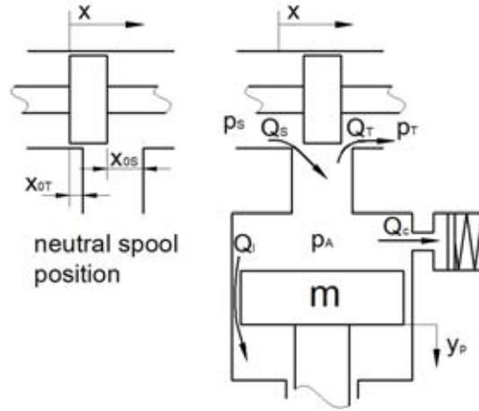
Fig. 3. Schema of hydraulic part of valve drive
