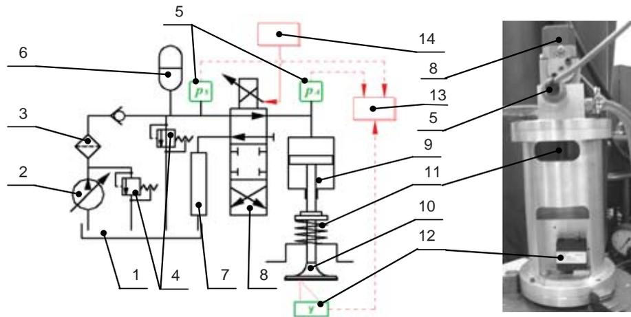
Fig. 5. Functional schema of electrohydraulic valve drive: 1 - tank, 2 - supply pump, 3 - filter, 4 - safety valves, 5 - pressure sensors, 6 - hydropneumatic accumulator, 7 - cooler, 8 - servovalve, 9 - actuator, 10 - engine valve, 11 - valve spring, 12 - position sensor, 13 - acquisition system, 14 - generator
