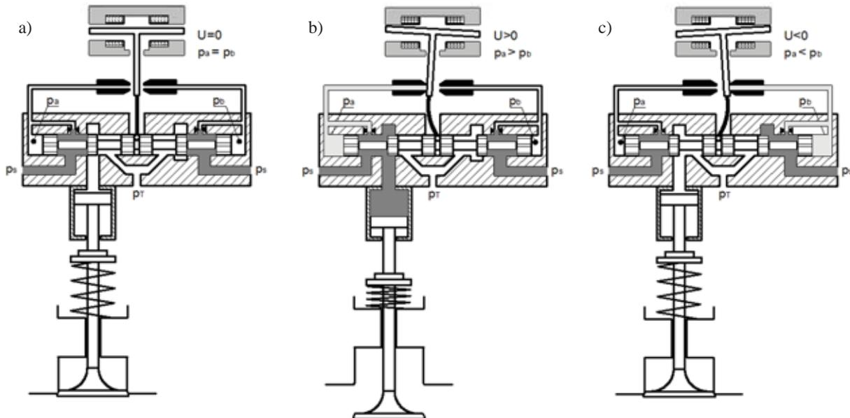
Fig. 2. The working phases of electrohydraulic valve drive
