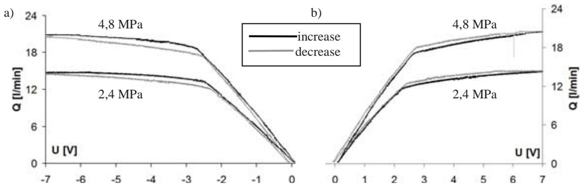
Fig. 6. Flowrate characteristics of servovalve: a) the outflow from the actuator b) the inflow to the actuator
