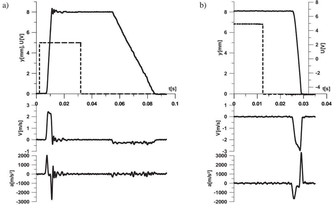
Fig. 7. Valve displacement, velocity and acceleration: a) return orifice opening equal the spool overlap, b) full opening of return orifice
