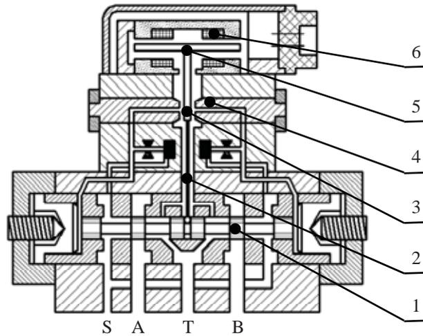
Fig. 1. Schema of Rexroth's servovalve type 4WS2EM10: 1- spool 2 - feedback spring, 3 - nozzle, 4 - flapper, 5 - armature, 6 - coil, S - inlet port, A - port A, B - port B, T - return port
