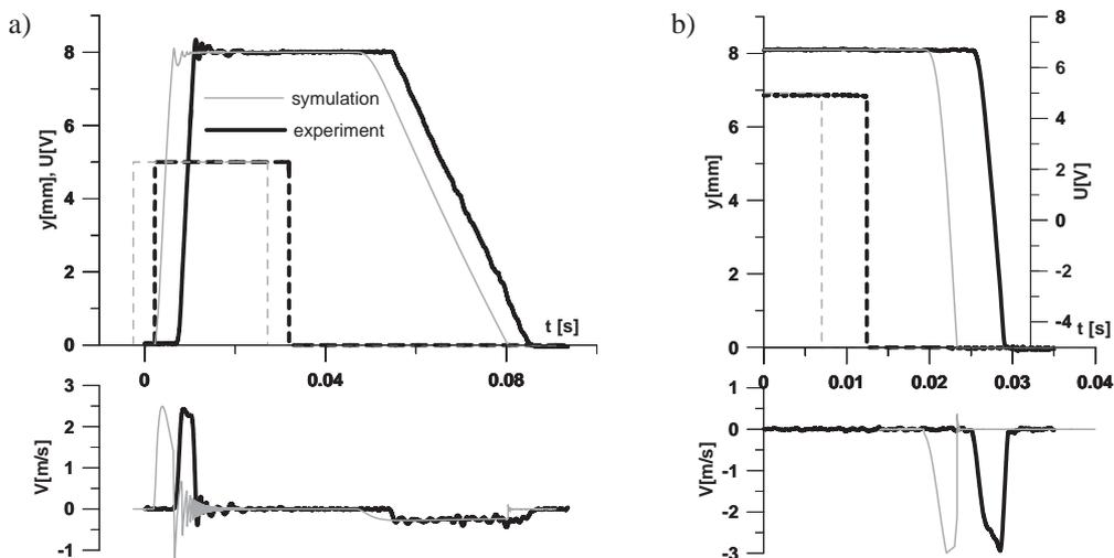
Fig. 8. Valve displacement, velocity and acceleration – test dates obtained from simulation and experiment: a) return orifice opening equal the spool overlap b) full opening of return orifice
