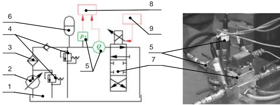
Fig. 4. The test stand for servovalve researches: 1 - tank, 2 - supply pump, 3 - filter, 4 - safety valves, 5 - pressure and flowrate sensors, 6 - hydropneumatic accumulator, 7 - servovalve, 8 - acquisition system, 9 - generator
